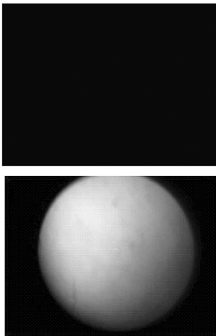
图 2 液晶盒的偏光照片:(a)暗态;(b)明态 Fig. 2 Polarized optical microscopic image of liquid crystal cells:(a) dark state; (b) bright state
